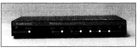
The KPC-9612 TNC is the centerpiece of Kantronics' packet paging system, with the latest release of the 9612 firmware supporting the mode. A personal computer may also be used to encode pager messages.
